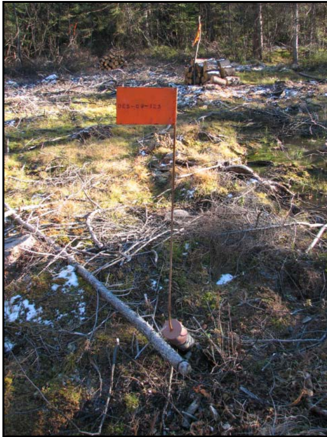
Figure 10.1 Diamond Drillhole Cap
